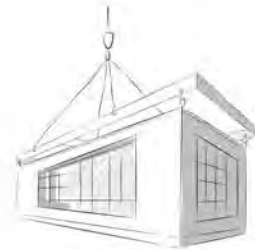
MEP systems, walls and glass are added.
