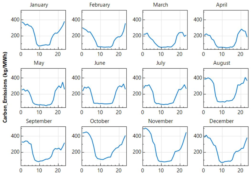
**Figure 21. Monthly profile of long-run carbon emission rates for end use loads (kgCO<sub>2</sub>e/MWh), by month, for the 2020 California Standard Scenario**
