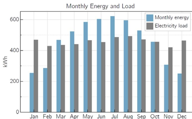
**Figure 23. Monthly energy consumption and energy generation of the apartment unit with 3.4-kWdc photovoltaic system. The excess energy generated by solar in the summer months balances the difference in energy consumption throughout the year.**
