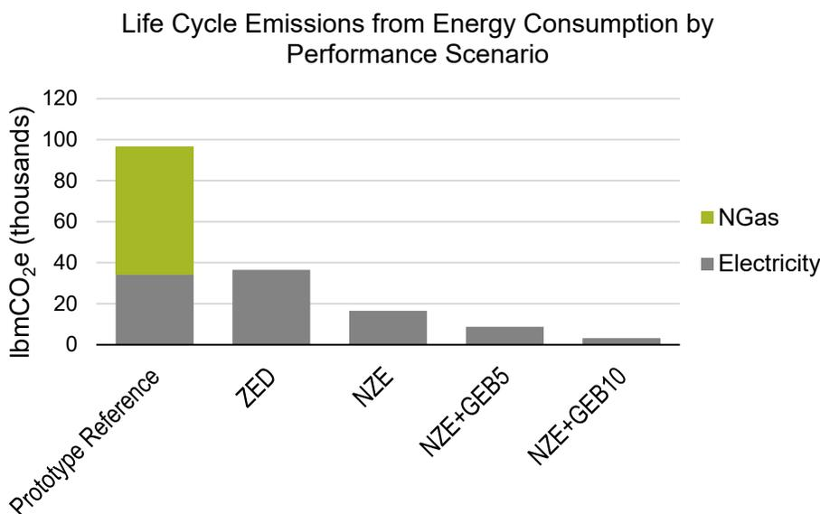
**Figure 9. Carbon emissions from building energy use over 30 years across five performance scenarios considered: “prototype,” “zero energy design,” “net zero energy,” “net zero energy plus grid-efficient battery 5 kWh,” and “net zero energy plus grid-efficient battery 10 kWh”**
