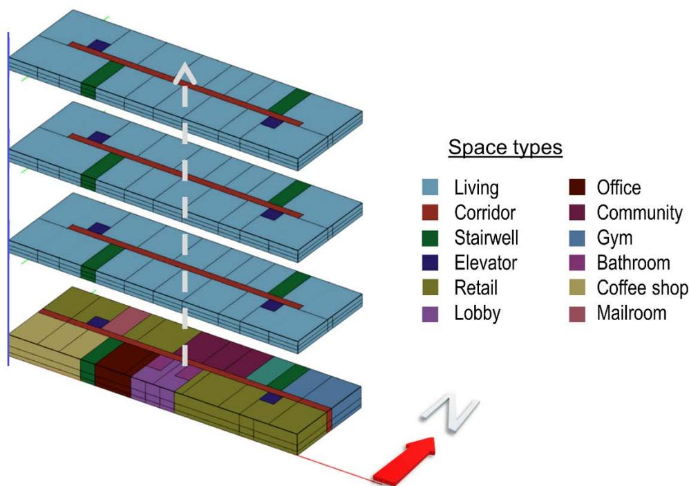
**Figure 16. Prototype multifamily model geometry by floor**
